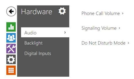
**2N** Indoor Talk is equipped with a speaker. This configuration section helps you set the phone call volume and state signalling volume. Master volume controls the general device volume including call volume, signalling tone volume, and so on. Consider the noise level of the ambient environment while setting this parameter.
