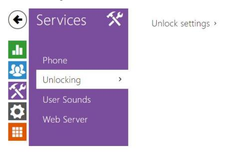
**Unlocking** is another function of **2N**<sup>®</sup> **Indoor Talk**, which sets the remote door unlocking parameters.
