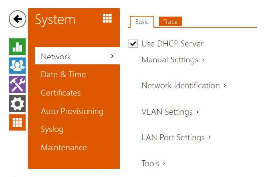
**2N** Indoor Talk is connected to the LAN and has to be assigned a valid IP address or obtain the IP address from the LAN DCHP server. The Network section helps you configure the IP address and DHCP.
