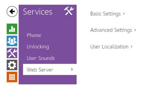
**2N**<sup>®</sup> **Indoor Talk** can be configured using a common browser that approaches the web server integrated in the device. The HTTPS protocol is used for the browser - device communication. Enter the login user name and password first. The default values are **admin** and **2n** respectively. We recommend to you change the default password as soon as possible.
