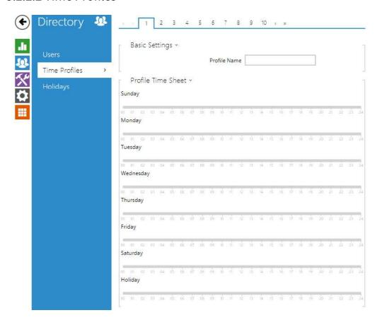
Such intercom functions as outgoing calls and RFID card/numeric code access, for example, can be time-limited by being assigned a **time profile**. By assigning a time profile you can:
