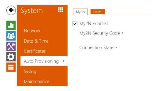
The **2N** Indoor Talk help you update firmware and configuration manually, or automatically from a storage on a TFTP/HTTP server selected by you according to predefined rules.
