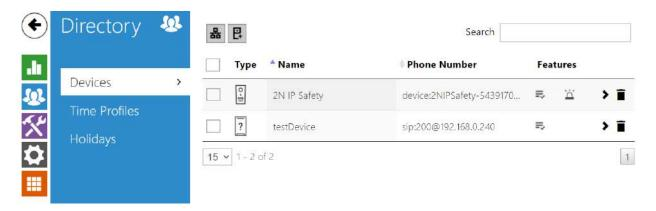
Directory is one of the crucial parts of the device configuration. It helps add new devices (2N IP intercoms and other answering units) and provides essential information on them. Up to 99 devices can be added to the directory.
