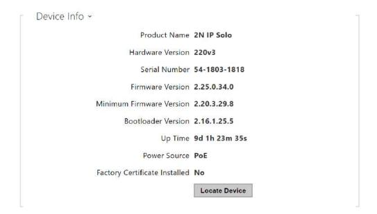
• **Factory Certificate Installed** – specify the user certificate and private key to validate the intercom right to communicate with the ACS.
