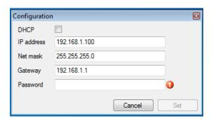
**2N® IP Network Scanner** IP Address Change
