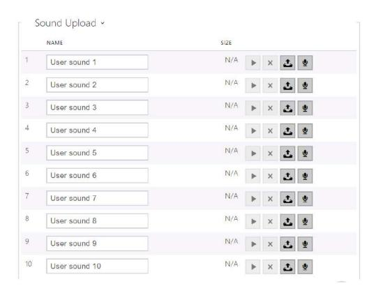
You can load up to 10 user sound files to the device and name each of them for better orientation.
