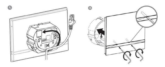
Remove the cover from the walled-in **2N**<sup>®</sup> **Indoor Talk** flush mounting box. Remove the prepared cabling, UTP cable, doorbell twin cable and power supply cable. Shorten the cables to 150 mm or less as required. Connect the doorbell twin cable or power supply cable to the connector provided. Crimp the RJ-45 connector onto the UTP cable.
