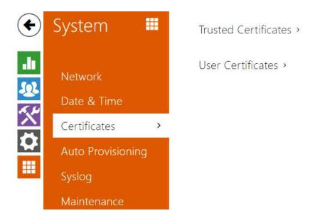
Some **2N**<sup>®</sup> **Indoor Talk** LAN services use the secure TLS protocol for communication with the other LAN devices. This protocol prevents third parties from eavesdropping on or modifying call contents. TLS is based on one/two-sided authentication, which requires certificates and private keys.
