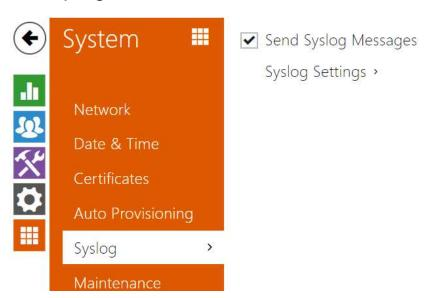
**2N**<sup>®</sup> **Indoor Talk** allows you to sends syslog messages including relevant device state and process information to a syslog server for recording and further analysis or auditing of the device observed. it is unnecessary to configure this service for common operations.
